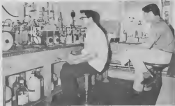
Lab Assistant Virgilio Angela (left) datamines nitrogen in HDS components with Kjeldahl distillation apparatus. At right, Lab Assistant Alberto Peña makes analysis of catacarb and MEA solutions using the automatic titrometar. Virgilio Angela (robaz) ta datamina nitrogeno den componentes di HDS cu aparato Kjeldahl di distilacion. Na drachi, Alberto Peña ta haci analisis di solucion catacarb usando titrometar.
